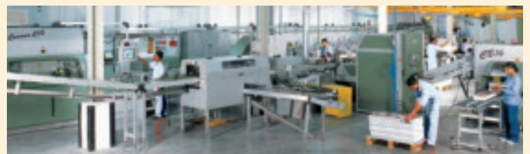
Our Muller Martini binders are JDF enabled and are connected to our Technique MIS system for automatic setting-up of jobs. They are also equipped with the Asir 3 automatic signature image recognition system to monitor and avoid any wrong upside forme being fed.
