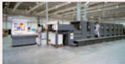
Our presses are connected with TECHKON and XRITE inline print density control systems for closed loop colour control to maintain colour density to FOGRA standards throughout the print run. All our presses are connected with Pre-press to receive CIP4 files for precise colour setting and job details. They are also connected with our Technique MIS system to plan and monitor the production schedule and optimise the whole printing process.
